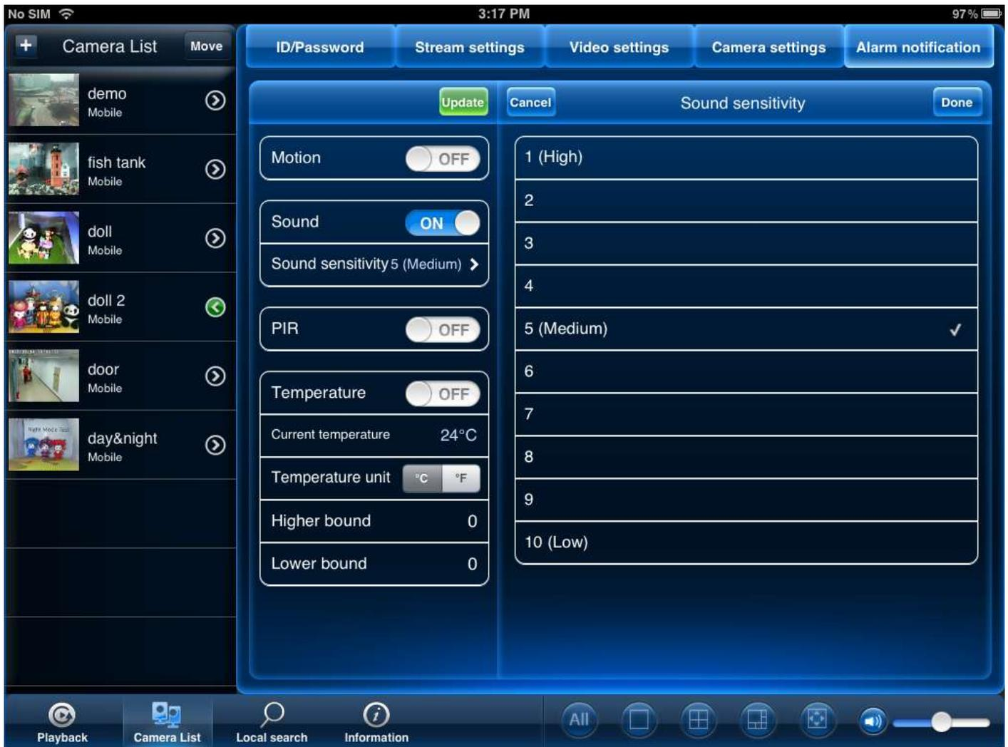
Push Alarm Notifications can be set up to create a notification straight to your iPhone when motion or sound is detected by the camera. Push Alarm Notifications go directly to the notifications area on your device.
